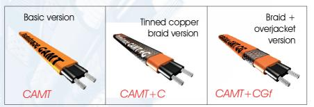
Do not use the CAMT heating cable on plastic pipe. It is imperative to comply with FIQ93 operating instructions. Warranty maxi exposure temperature : power ON = 85°C / power OFF 125°C. Maximum maintenance advised temperature : 65°C. Beyond these exposure temperatures use control thermostat.
